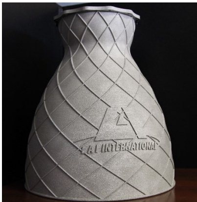
Figure 1: Nozzle as Printed
