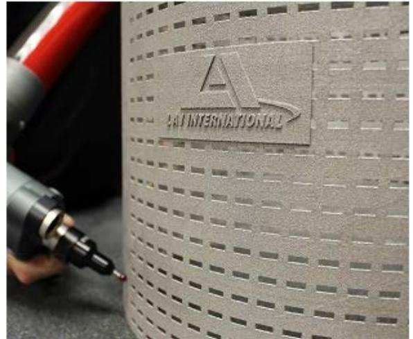
Figure 1. Intermediate dimensional checks ensure conformance to requirements before additional post-processing steps commence. Photos courtesy of LAI International.
