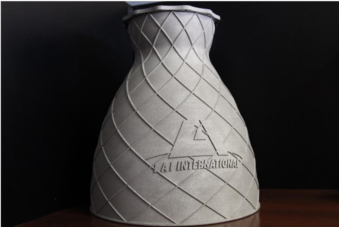
Figure 3. A large nozzle was built to demonstrate the size potential of LAI's electron beam powder bed fusion technology.
