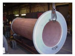
For VAR melters, limited to round static ingot crucibles with standard taper, the hoop strength of the round coupled with the external stiffeners should render even more impressive results. We would not be surprised with 2500-3000 heats before resizeing required. On that basis, amortized crucible costs would be expected to drop to below .5 cents per product pound.
